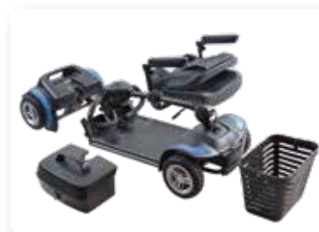
Easily disassembled into five pieces
