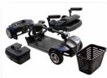
TK-056: easily disassembled into five pieces
